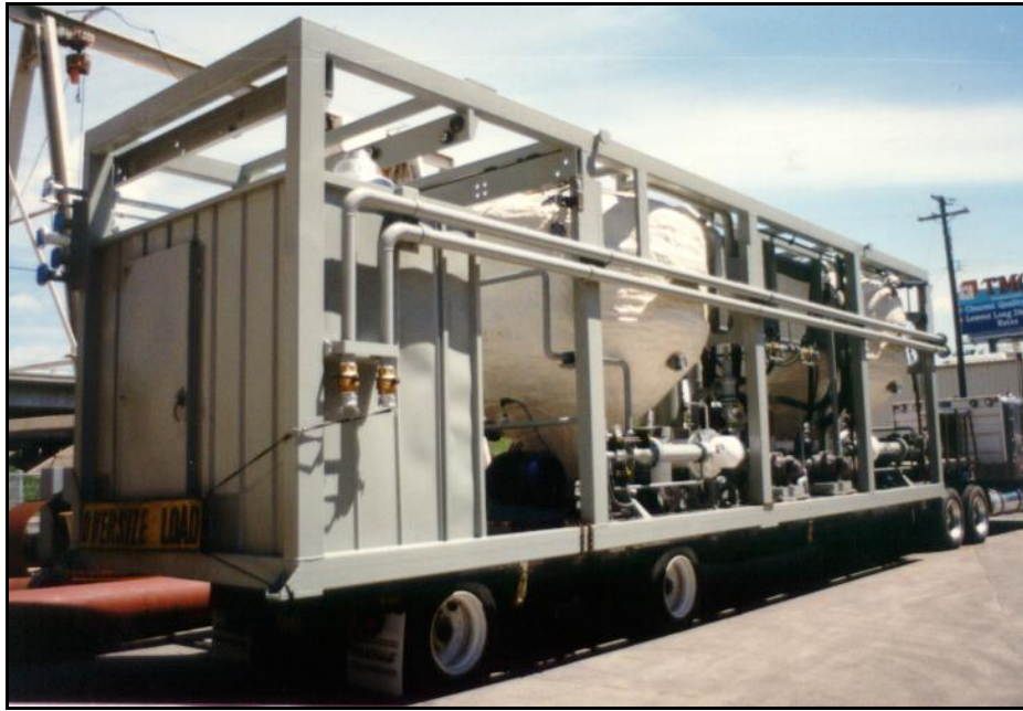
Photo #7. Factory tested module unit ready for shipment.
