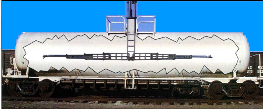
Pic. 2. Extended and unfolded telescopic apparatus inside car.
