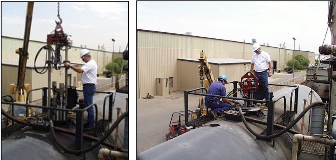
Photo #6. Telescopic apparatus installation on the car manway.
