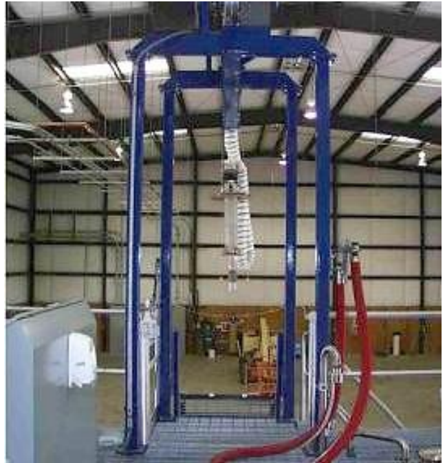
Photos 3a and 3b. Manway adapter installed on in top manway of tank trailer and adjustable gangway platform for installation of manway adapter.
