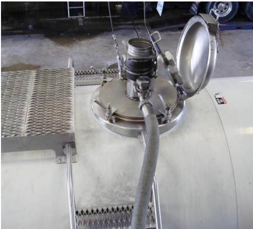
Photos 3a and 3b. Manway adapter installed on in top manway of tank trailer and adjustable gangway platform for installation of manway adapter.
